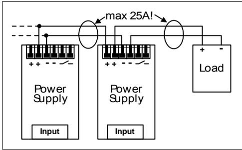
Fig. 27-7 Using distribution terminals
