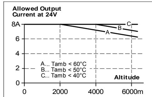
The ambient temperature is defined as the air temperature 2cm below the unit.
