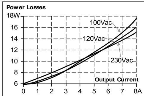
Fig. 11-3 Efficiency vs. input voltage, 24V, 8A
