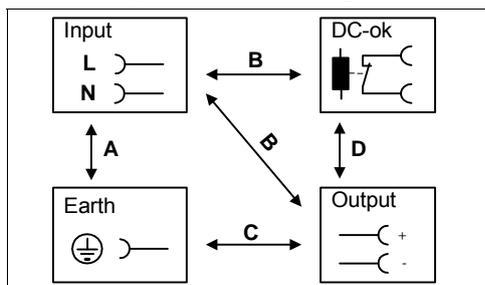
The output voltage is floating and has no ohmic connection to ground.
