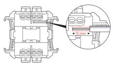
Type of terminals: automatic Terminal capacity: 1.5 mm<sup>2</sup> - 2.5 mm<sup>2</sup> (1 or 2 conductors) Stripping length: 13 mm
