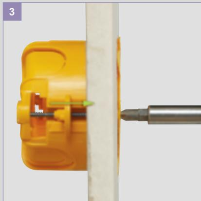
Fixing claws adapted to the thickness of the wall
