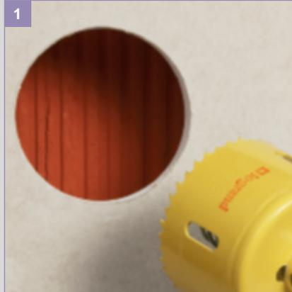
Hole cutter saw Ø67
