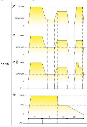
**Operating mode without memory:** at switch-off, the light level is not memorized.
