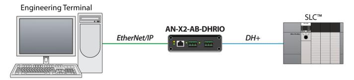
This operating mode acts as a bridge between an EtherNet/IP and a Data Highway Plus network.
