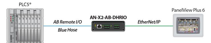
This operating mode allows legacy PanelViews on Remote I/O to be upgraded to a PanelView Plus or a PanelView Plus 6 on EtherNet/IP.
