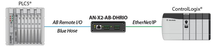
This operating mode allows PLC's on Remote I/O to share data with a newer ControlLogix or CompactLogix PAC's. This mode also allows a ControlLogix processor to monitor Block Transfer and I/O data on an active Remote I/O network without occupying a drop.
