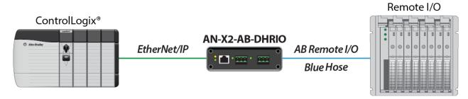
This operating mode allows users to replace their existing Remote I/O PLC with a ControlLogix or CompactLogix PAC without having to replace existing racks of I/O.
