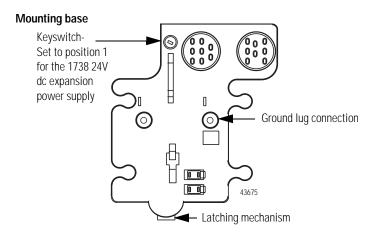
To remove the power supply from the mounting base:
