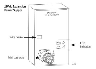
The 24V dc expansion power supply unit (Cat. no. 1738-EP24DC) passes 24V dc field power to the I/O modules to the right of the power supply. This unit extends the backplane bus power for up to 17 I/O modules to the right of the supply and creates a new field voltage partition.
