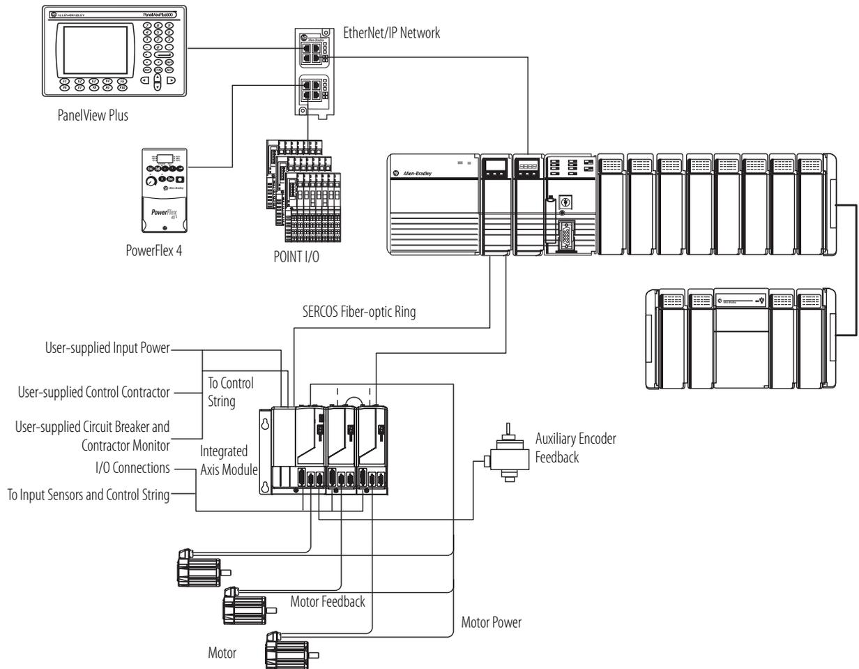
A three-axis system with Kinetix drives supports:
