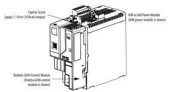
**6.** Repeat  $\underline{\text{step 2}}$  through  $\underline{\text{step 5}}$  to mount a control module onto each power module installed on your Bulletin 2094 power rail.
