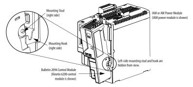
4. Pivot the control module toward the power module to engage the signal connectors and guide pins.
